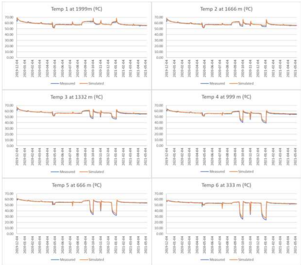
Figure 7 - Comparison of Measured and Simulated thermocouple data from Eavor-Lite™
